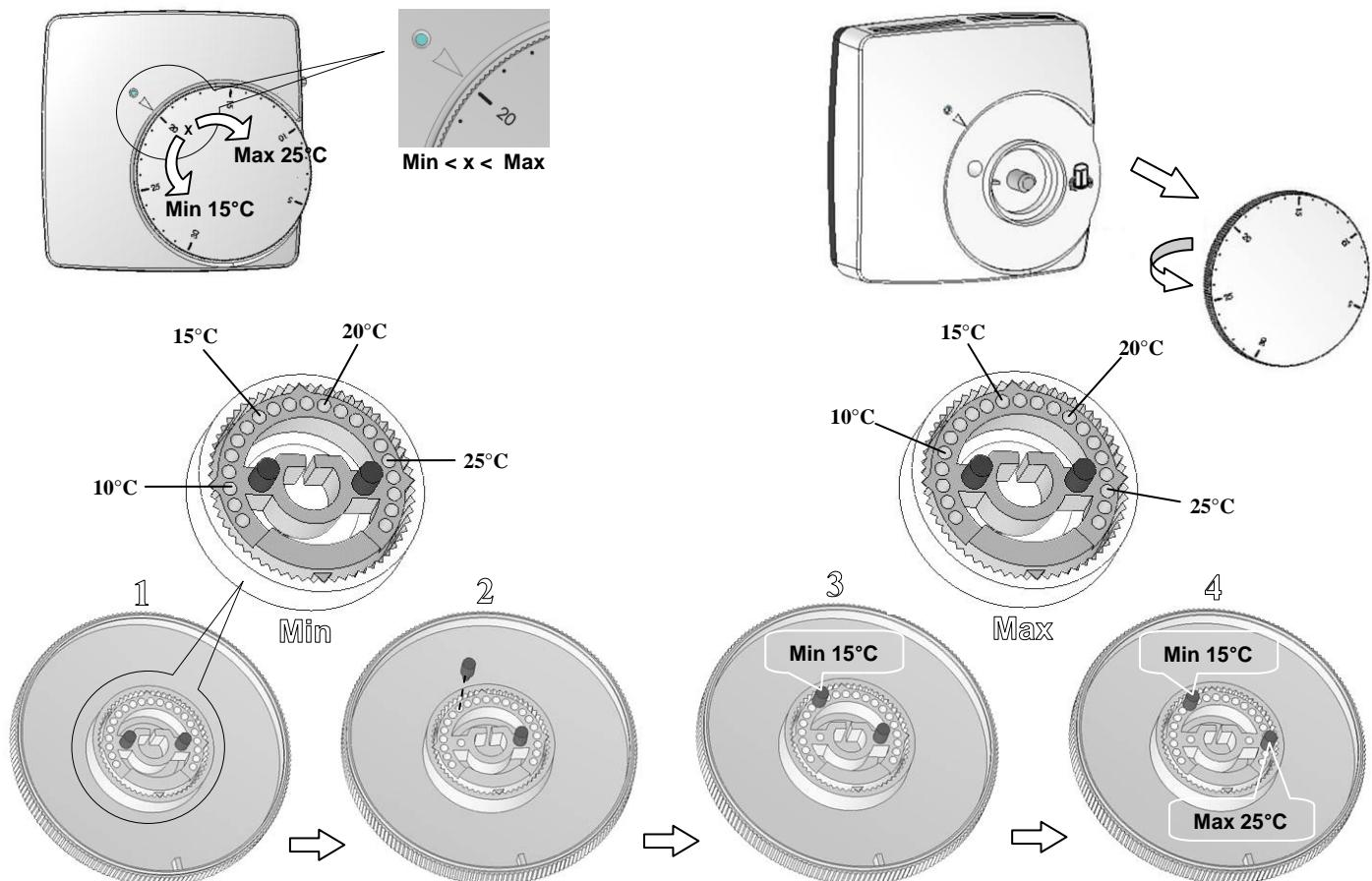
**D** Kalibrierung    **GB** Calibration    **F** Calibration    **E** Calibración    **I** Calibrazione
